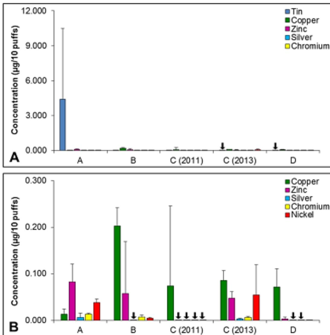
**Figure 2 Total concentration of metals in aerosol of four brands of E(N)NDS.**
