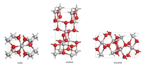
This figure shows the three structural forms of titanium dioxide- rutile, anatase and brookite. The image is red and grey on a white background and has 3 structural forms: rutile, anatase and brookite.
