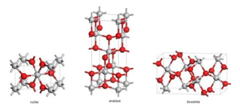
This figure shows the three structural forms of titanium dioxide- rutile, anatase and brookite. The image is red and grey on a white background and has 3 structural forms: rutile, anatase and brookite.
